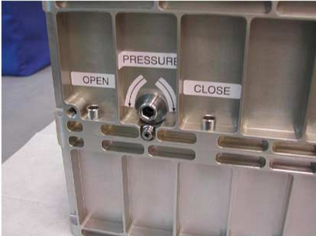
Figure 4-15 : Detail view of the depressurization screw. This screw is fitted internally with two separate viton o-rings. It is captive due to the presence of the locked second screw (small one below)
