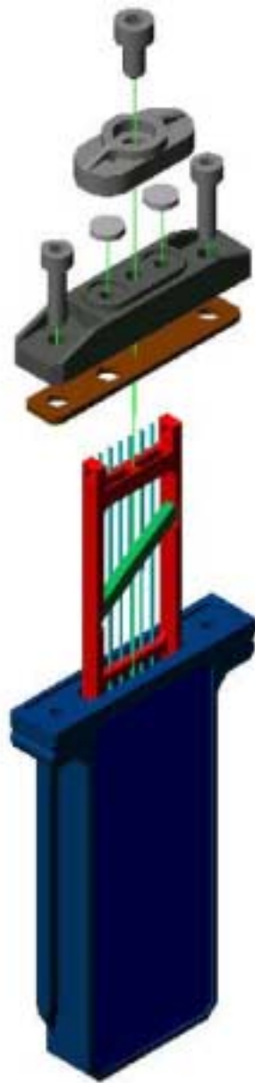
Figure 4-5: PROMISS experimental cell (exploded view)
