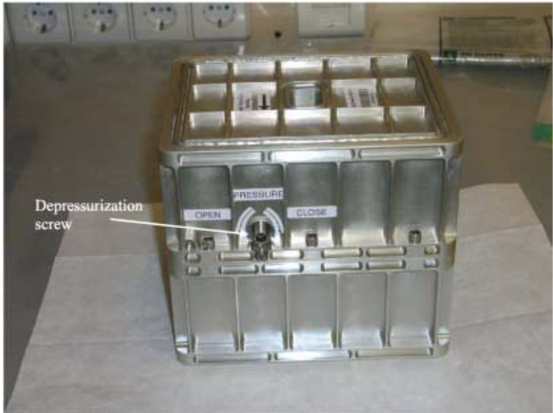
Figure 4-14 : PROMISS Sample Container fitted with the depressurisation screw.
