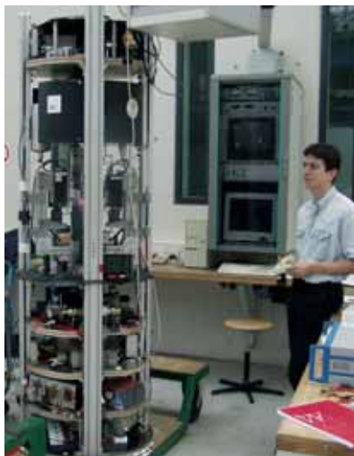
Preparing the experiment 'Soot Particle Growth of a Diffusion Flame' using laser-induced incandescence.
