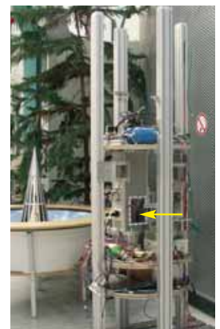
The set-up for studying how materials burn in space. The windtunnel (arrowed) simulates typical airflow aboard the Space Station.
